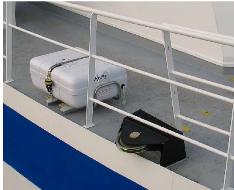
Figure 2-12 Stbd Upper Deck - Liferaft & Warp Cable Block
