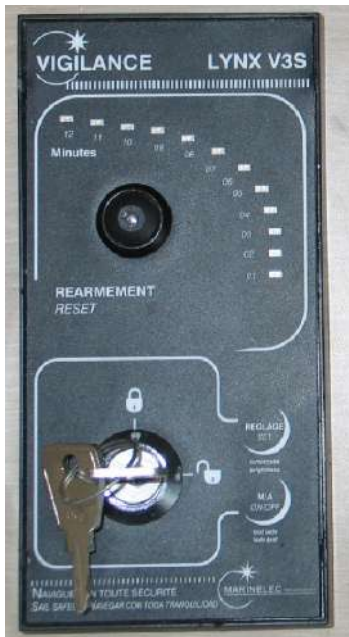
Figure 5-33 Bridge - Navigational Watch Alarm
