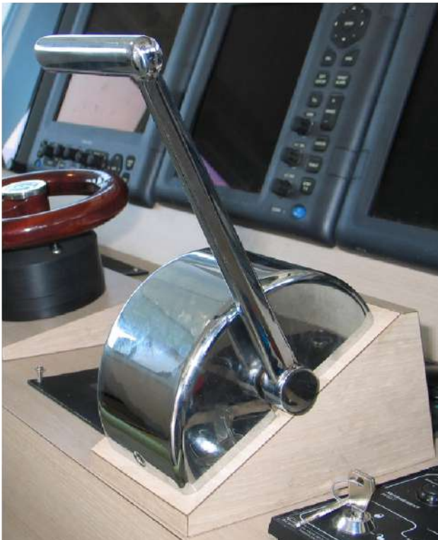
Figure 5-37 Bridge Mechanical Control Head
