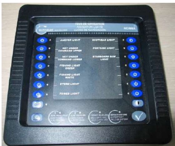
Figure 5-34 Bridge - Navigation Lights Monitoring & Control Panel
