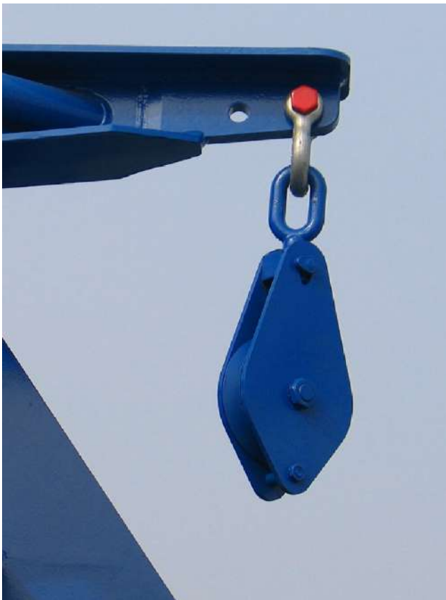
Figure 2-11 Gantry - 6 Tons Warp Block
