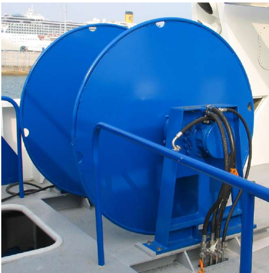
Figure 2-8 Portside Upper Deck - Single Net Drum
