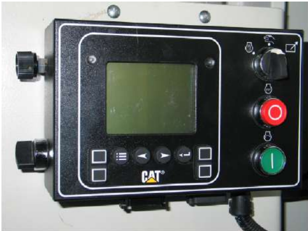
Figure 5-35 Bridge - MECP-1 Engine Control Panel
