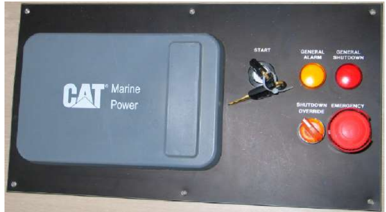
Figure 5-36 Bridge - Engine Remote Control Panel
