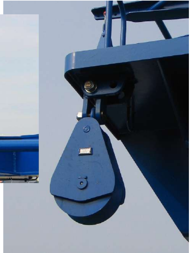
Figure 2-10 Gantry - 15 Tons Warp Block
