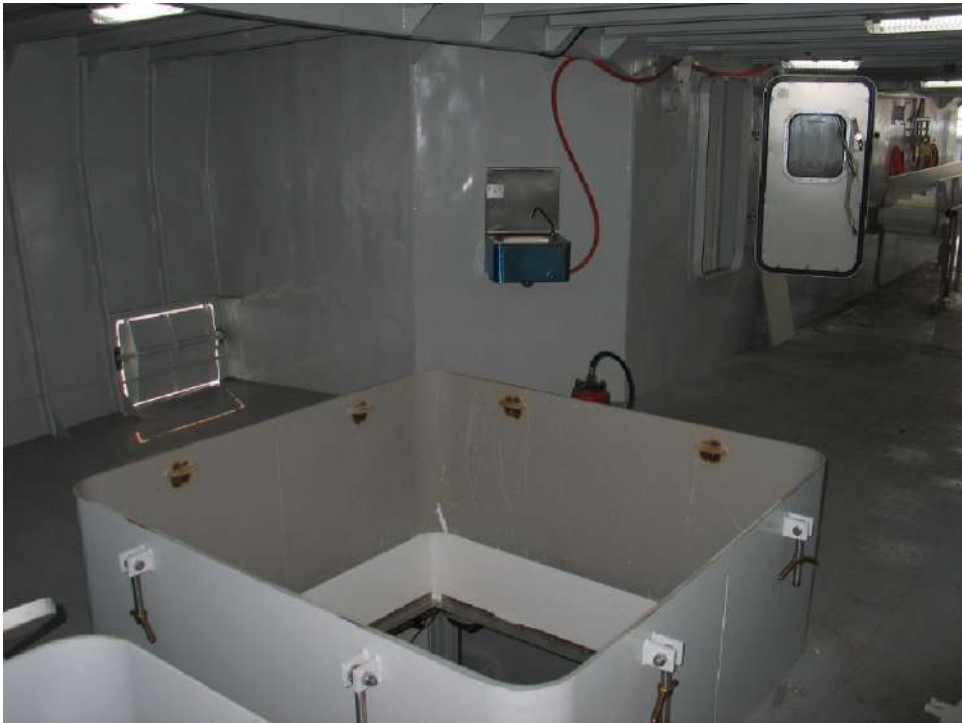
Figure 2-37 Fore Fishing Deck - Fish Hold Hatch
