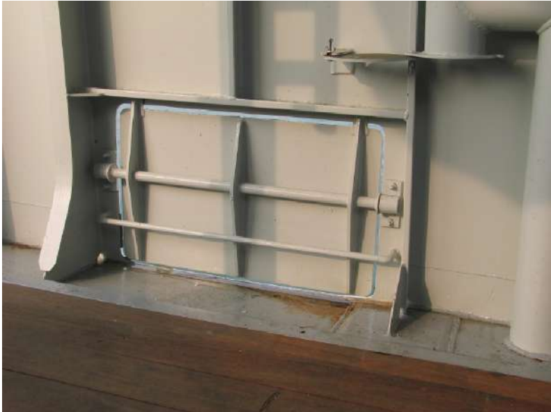
Figure 2-36 Fishing Deck - Aft Port Freeing Port
